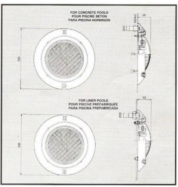
It includes cross shaped reinforced plastic fixing unit using plug, stainless steel screws & gaskets
