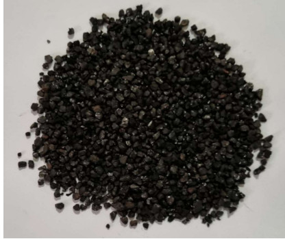
Figure 4, Granular Activated Carbon
